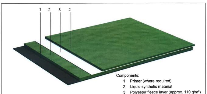
Applicable to the roof waterproofing " DAKORIT PUR 1K 30P "
